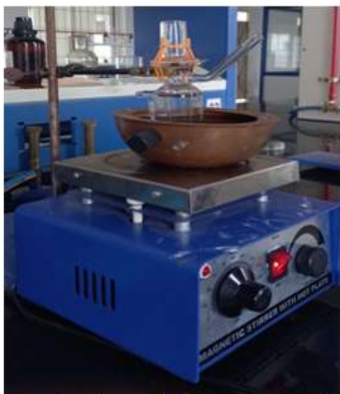
Fig 2: Franz diffusion cell with magnetic stirrer
